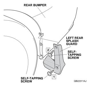
14. Secure the bottom of the left rear splash guard to the rear bumper with one self-tapping screw supplied.
