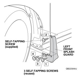
5. Turn the steering wheel fully clockwise, and repeat steps 2 through 4 to install the right front splash guard.
