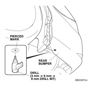
Install one spring nut A over the scribe mark of the rear bumper. Using a washer and self-tapping screw, secure the spring nut A to the rear bumper as shown.
